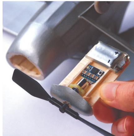
Access is required to the Zombie to alter the 'trim pots' and to hit the on/off switch. To eliminate the need for hatches we recommend the use of a slide-out tray built into the model (see picture of Keil Kraft Luscombe Silvaire right). This system has many advantages: The Zombie's switch and pots can easily be operated, the self-contained tray is easy to wire up and
